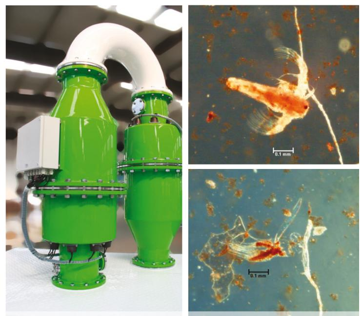
Microorganisms before (above) and after treatment within the system reactor unit.
